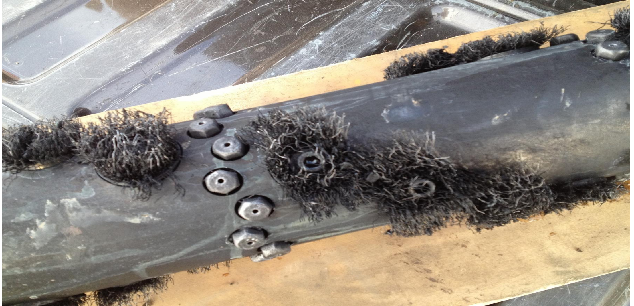
Condition of replaceable wire brushes after a well cleanout
